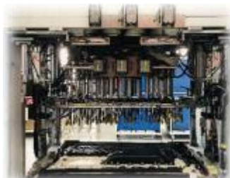
热铆焊接 Hot Riveting Welding
